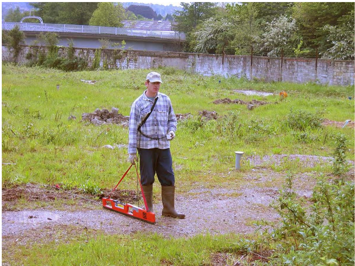
Figure 1: Ground Conductivity instrument being used to locate buried foundations
