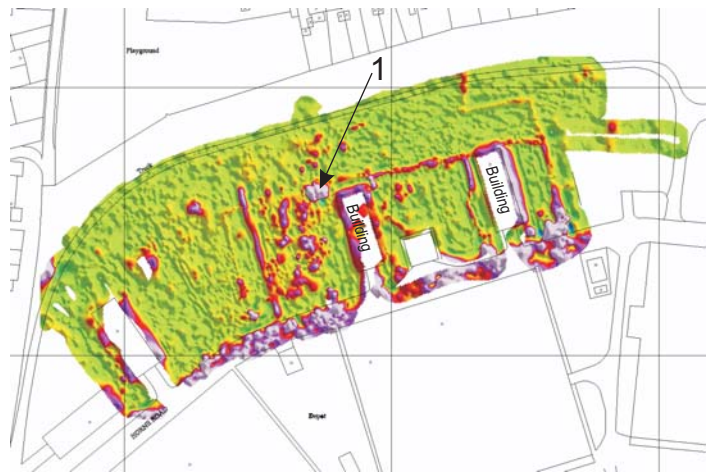
(ABOVE) Processed magnetic data from a former industrial site showing linear anomalies from ferrous buried services. The isolated magnetic anomaly marked "1" was ground truthed to be an underground fuel tank. (Note the magnetic effect of the buildings).
