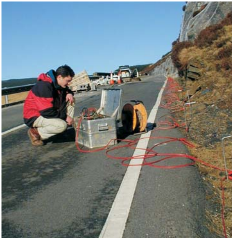
resistivity cable deployment in road verge
